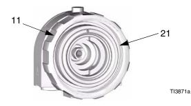
2. Orient front end as required for desired fluid manifold mounting (bottom mounting shown). Align slots (Y) to engage tabs (Z).
