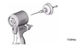
**9.** Install piston safety lock assembly until bottomed out.
